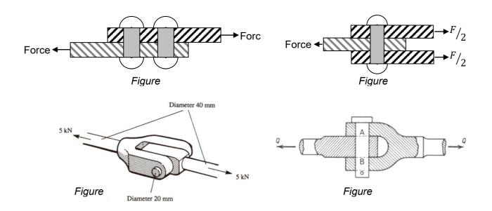
Discuss and compare the advantages and limitations of single shear (Figure A) and double shear riveted joints (Figures B, C, D and E). Within your discussion compare and contrast joints using single and double shear arrangements in addition to using typical worked numerical examples to validate key areas of your discussion.
